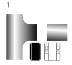
The cut ends of the pipe should be smooth and square.
