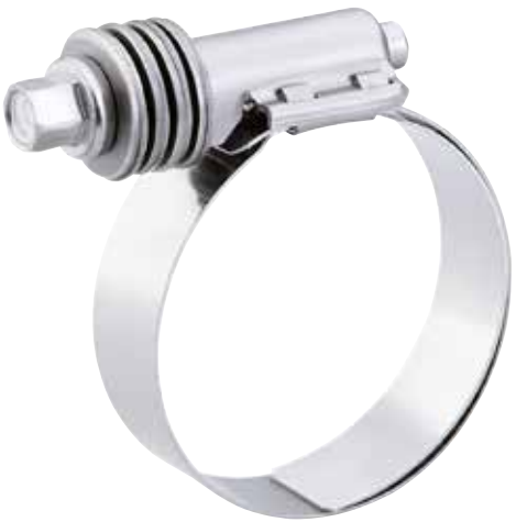
Constant-Torque - Aero Seal Construction Per SAE standard J1508 Type “SLF”
